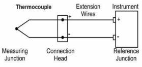
A **thermocouple** is a sensor for measuring temperature. This sensor consists of two dissimilar metal wires, joined at one end, and connected to a thermocouple thermometer or other thermocouplecapable device at the other end. When properly measurements over wide range of temperatures.
