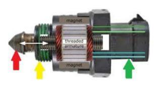
This image shows the inner workings of a typical Idle Air Control valve. In this example, the red arrow indicates the valve pintle, the yellow arrow indicated the threads that mount this particular example on the throttle body, and the green arrow indicates the electrical connector.
